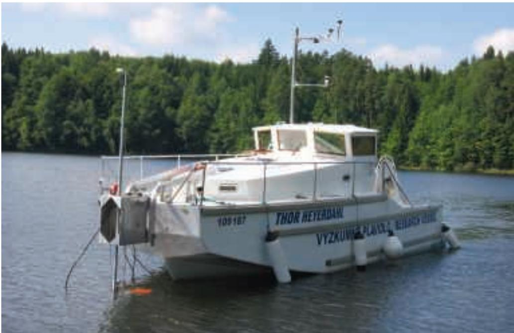
**Fig. 4.2.1.** Transducers in the fore part of the research vessel exploring the reservoir (photo: FISHECU archive).
