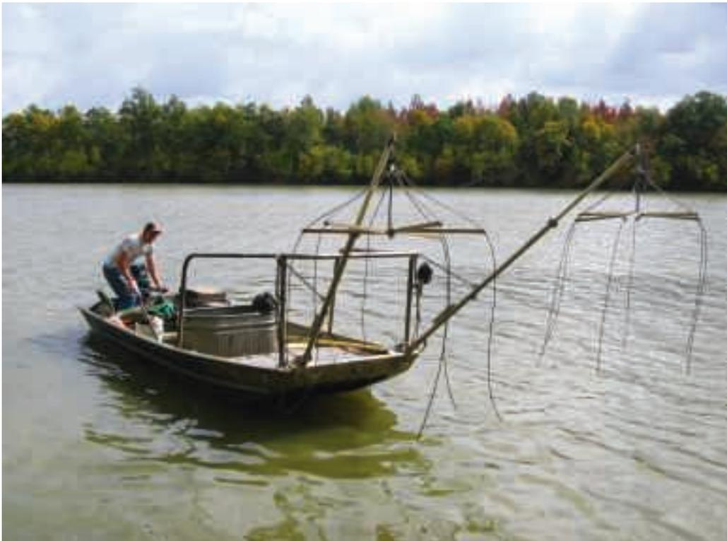
**Fig. 6.1.4.** An electrofishing boat with a safety railing and a system of two anodes placed obliquely in front of the vessel's hull (Smith-Root, USA) (photo: M. Kratochvíl).
