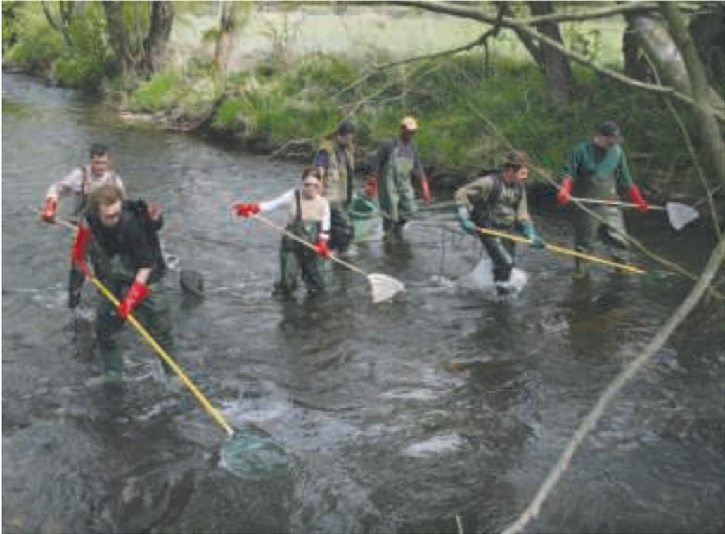
**Fig. 6.1.3. Electrofishing using two backpack electrofishing devices in a medium size stream** (Blanice River, Vodňany; photo: M. Bláha).
