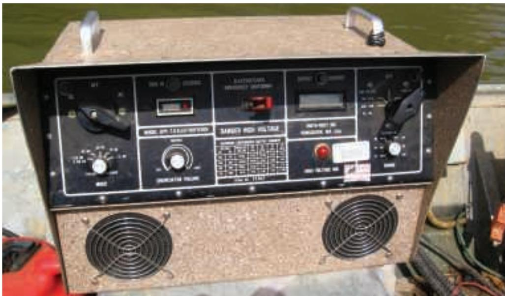
**Fig. 6.1.6.** A stand-alone power unit with options of setting parameters of the type of electrical current, settings of voltage, frequency, working cycle, etc. (Smith-Root, USA) (photo: M. Kratochvíl).
