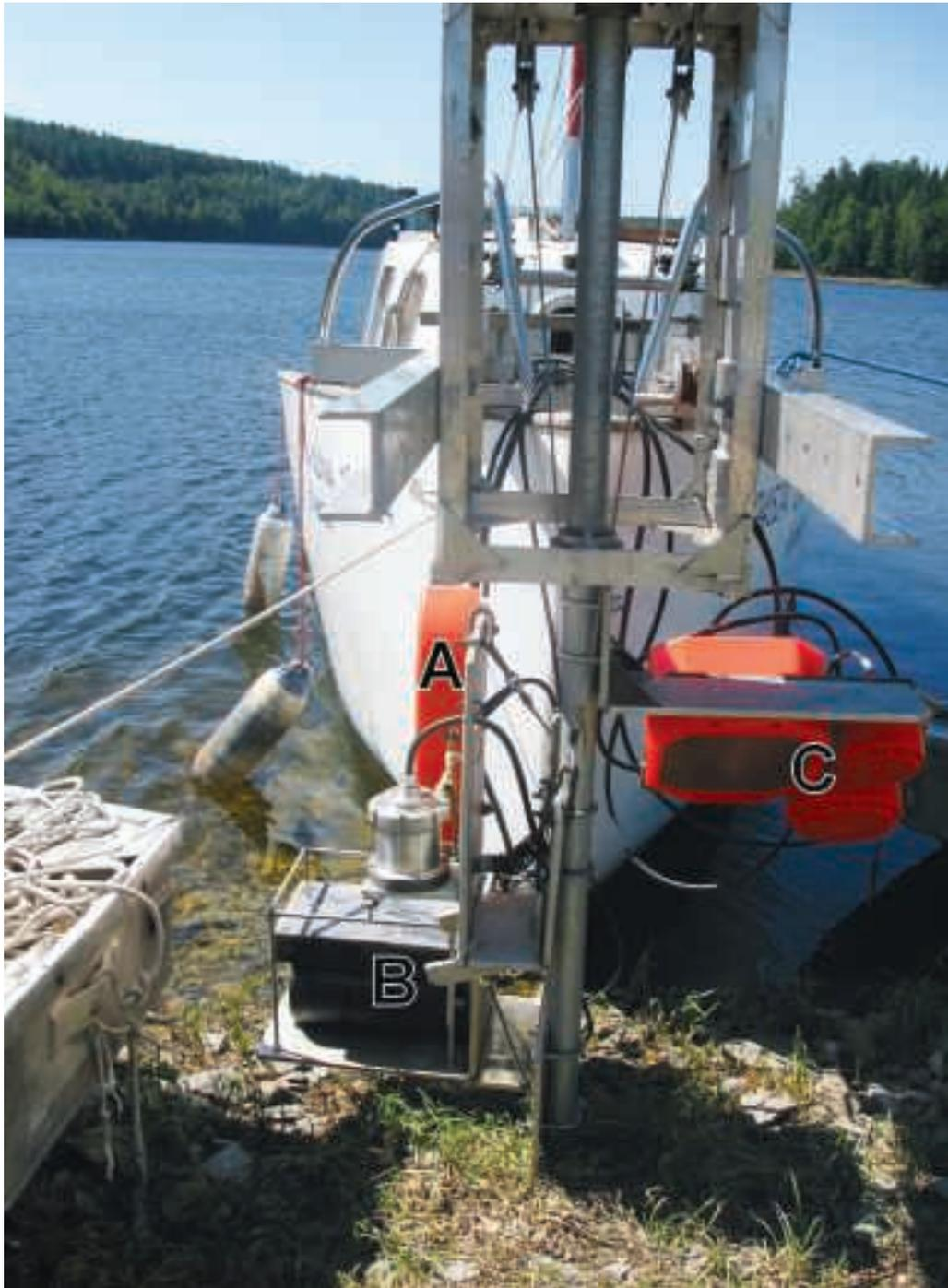
**Fig. 4.2.2. Transducers in the fore part of the research watercraft.** A: Elliptical 120 kHz transducer for horizontal “beaming”; B: Didson acoustic camera, C: Transducers for vertical surveying: 38, 120 and 400 kHz (photo: FISHECU archive).
