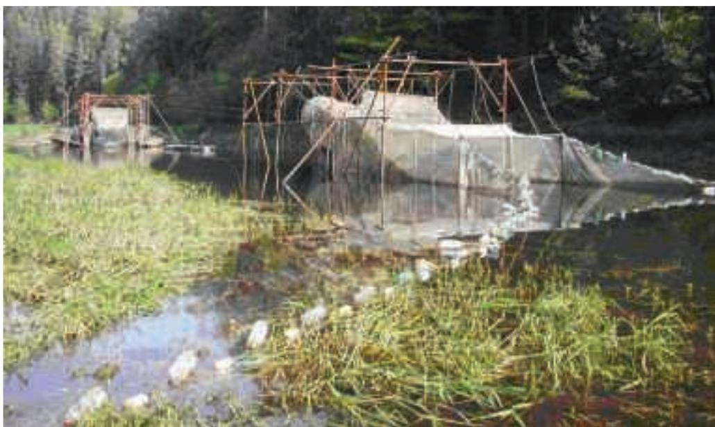
**Fig. 4.7.3.** The system of two large fyke nets installed across the inflow zone at the Římov Reservoir. With respect to the dimensions of the chamber and the size of catches, it was necessary to build scaffolding in order to set and manipulate each trap (photo: FISHECU).
