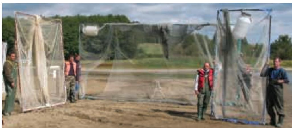
**Fig. 6.2.6.** Frame ichthyoplanktonic trawl used for catches of the earliest stages of fry in open waters of dam reservoirs (above, photo: P. Pokorný) and fry trawls used for catching juvenile fry later in the season (below, photo: FISHECU).
