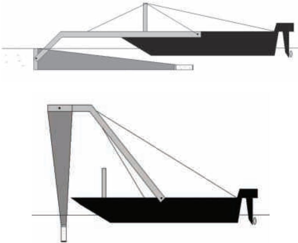
**Fig. 6.2.8.** Sketch of a net pushed in front of a vessel during sampling (top) and positions of the push net after sampling completion before emptying the catch (below, according to Herzig et al., 1994).
