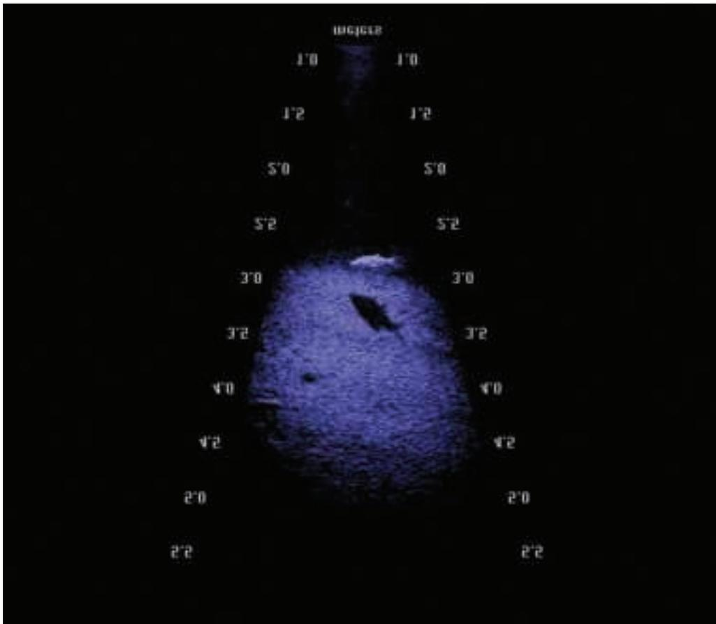
**Fig. 4.2.5.** Bream in the Elbe River on the record of a DIDSON multi-beam acoustic camera. The view is inclined from the water surface towards the bottom and it is possible to see the fish and its shadow on the bottom approximately 3 m from the camera (photo: M. Tušer)
