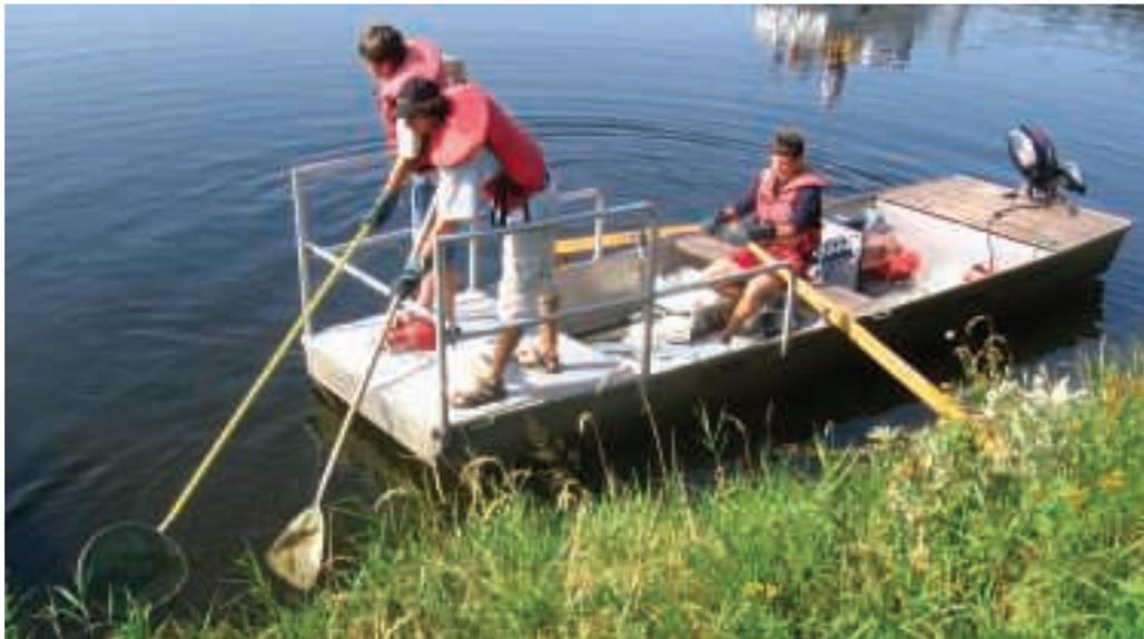
**Fig. 6.1.8. Catching of fry from boats using point sampling.** The positive anode (circular shape) at the end of the fibreglass rod is placed into the water in front of the boat and at the same time the electric field is activated. All stunned fish are then collected by a catcher with a landing net (photo: M. Kratochvíl).
